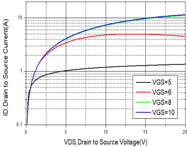
**Figure 1 Output Characteristics**
