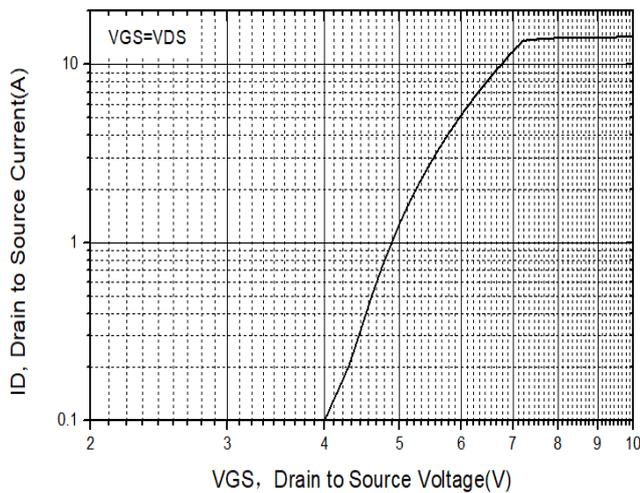
**Figure 2 Transfer Characteristics**
