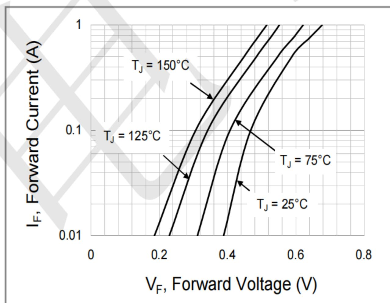
Fig.4 Typical Forward Characteristics
