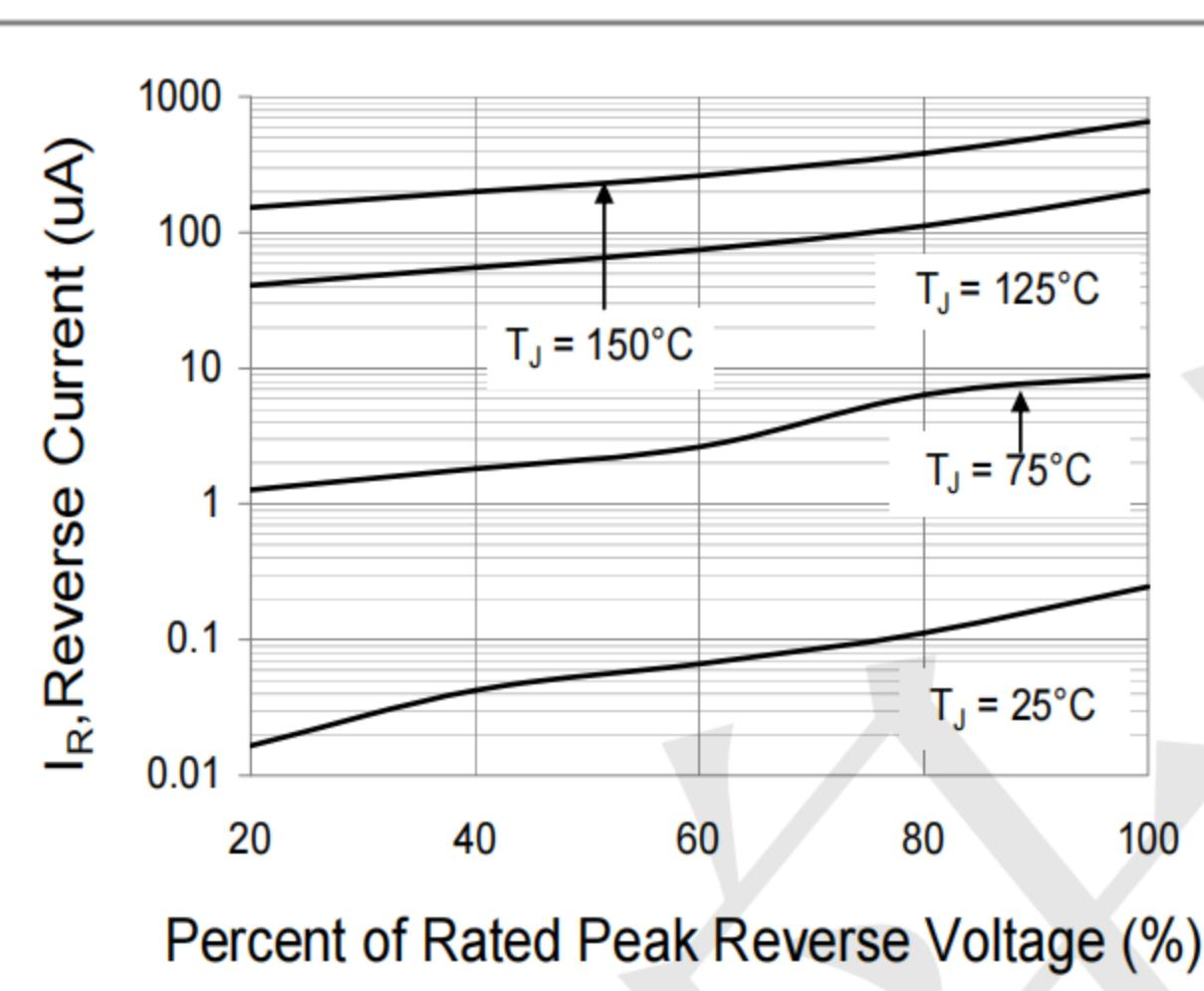
Fig.3 Typical Reverse Characteristics
