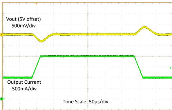
$V_{IN} = 3.3V$ ,  $V_{OUT} = 5V$ ,  $I_{OUT} = 1A$  至  $2A$ , 压摆率为  $20\mu s$
