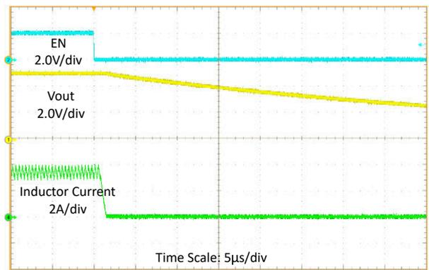
$V_{IN} = 3.3V$ ,  $V_{OUT} = 5V$ ,  $2.5\Omega$  电阻负载
