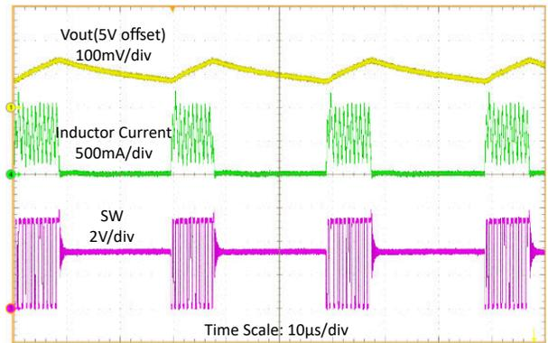
$V_{IN} = 3.3V$ ,  $V_{OUT} = 5V$ ,  $I_{OUT} = 100mA$
