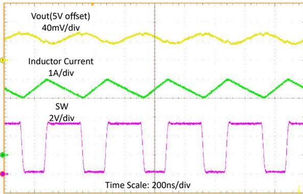
$V_{IN} = 3.3V$ ,  $V_{OUT} = 5V$ ,  $I_{OUT} = 2A$
