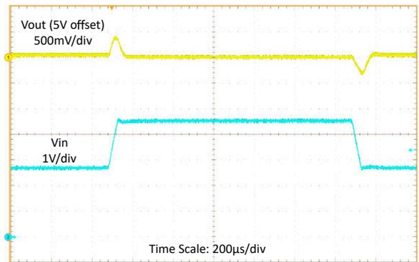
$V_{IN} = 2.7V$  至  $4.5V$ , 压摆率为  $20\mu s$ ,  $V_{OUT} = 5V$ ,  $I_{OUT} = 2A$
