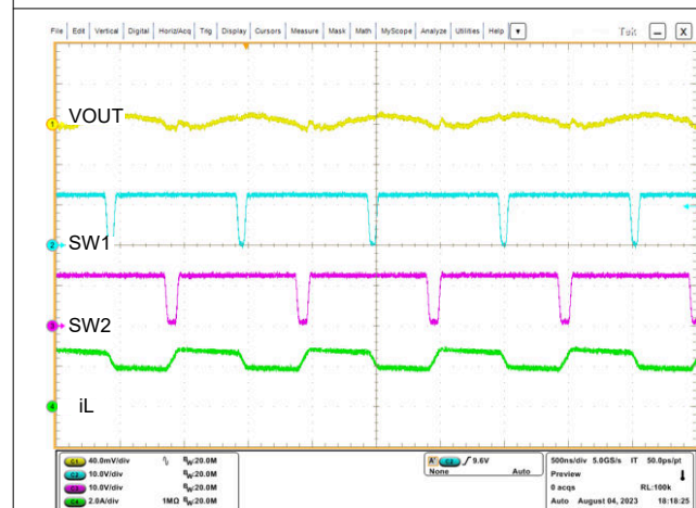
图 8-4. Switching Waveforms in V_{IN} = 12\text{ V} , V_{OUT} = 12\text{ V} , I_O = 2\text{ A} , FPWM
