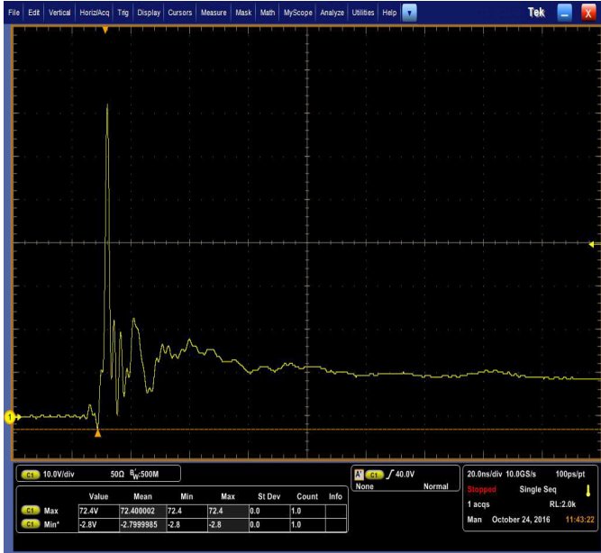
Figure 3. Positive 8kV contact per IEC 61000-4-2
