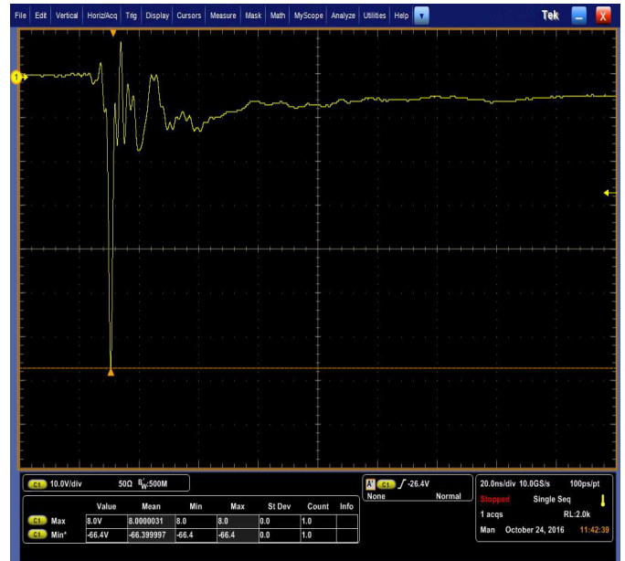
Fig 4. Negative 8kV contact per IEC 61000-4-2
